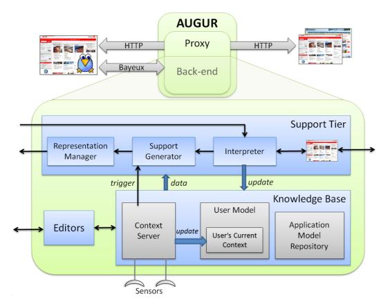
Figure 5.13. Architecture of the AUGUR prototype
