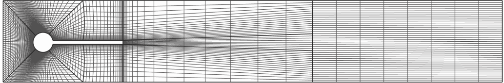
Figure 4.2: Coarse mesh for the fluid field, every second grid line is plotted
