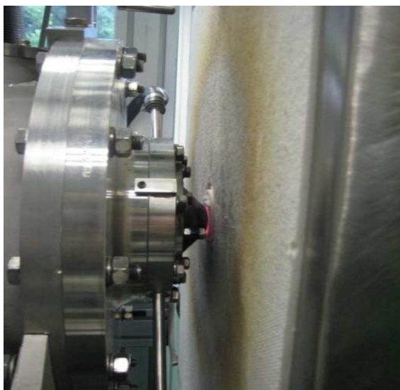
Figure 11. Flow channel furnace coupled with the MBMS.
