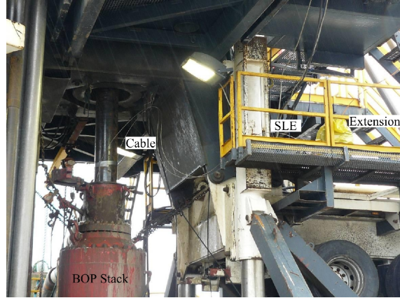
Figure 3.4.: Experimental Set-up during cementation of the anchor casing. The cable is feed through the BOP stack and the surface excess length is placed on the rig. The fibre optic extension is wrapped in a yellow plastic bag to keep it dry during the measurements.
