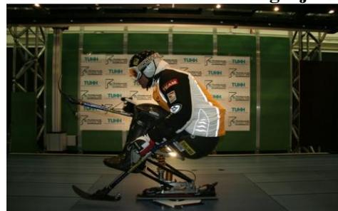
photo T2P4S1 – Drag Coeff. 0.254 10 m/s photo T2P4S1j – Drag Coeff. 0.307
