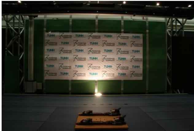
Fig. 21: Wooden plate adapted to skis and fixed to the 6 component balance.
