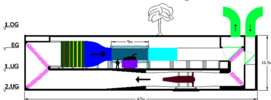
Fig. 19: Schematic View of the Wind Tunnel (<http://www.tu-harburg.de>).
