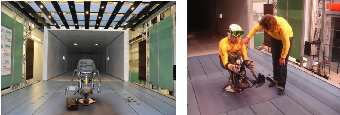
Fig. 20 (a, b): Frontal view from the test section; Seated mono-ski fixed to the balance.
