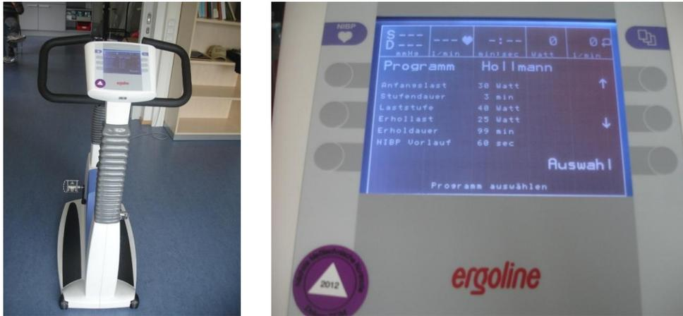
Fig. 16 (a, b): Ergoselect 200 electric bicycle ergometer; bicycle graphic display unit.
