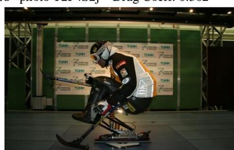
photo T2P4S3 – Drag Coeff. 0.252 30 m/s photo T2P4S3j – Drag Coeff. 0.326
