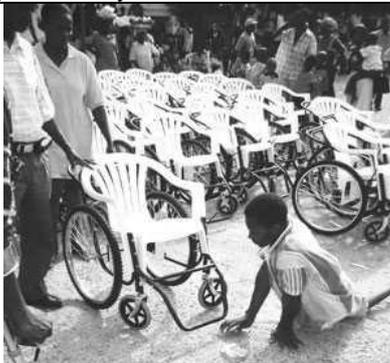
Fig. 42: WC developed by "Free Wheelchairs Mission".
