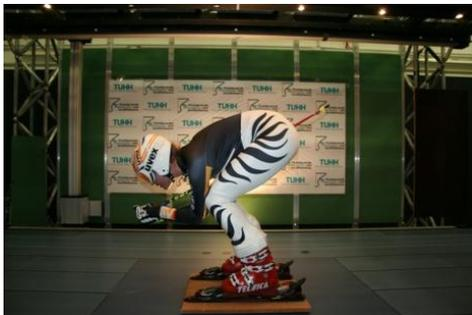
photo T2P1S2 – Drag Coeff. 0.182 20 m/s photo T3P1S2 – Drag Coeff. 0.195
