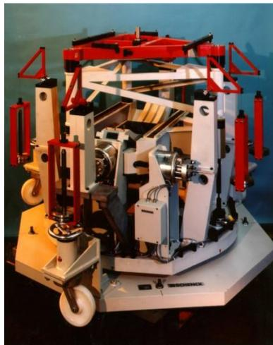
Fig. 22: Six-component (External) Balance (<http://www.tu-harburg.de>).
