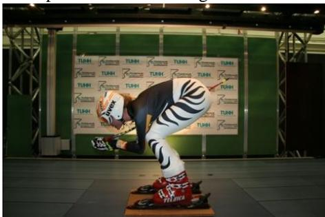
photo T2P1S3 – Drag Coeff. 0.178 30 m/s photo T3P1S3 – Drag Coeff. 0.184
