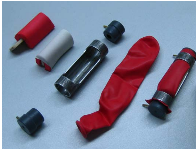
Figure 3.8 Assembling steps of the artificial lip. The air-balloon is subsequently filled with glycerin through tiny brass capillaries fitted in the PVC caps.
