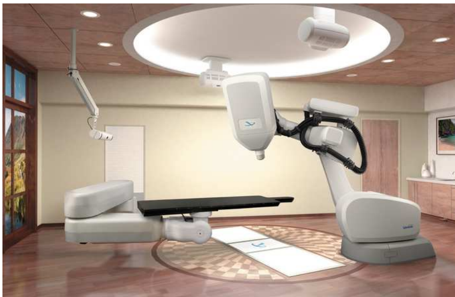
Figure 1.15.: Cyberknife Synchrony system. The linear accelerator is mounted on a robotic arm. Motion monitoring for mobile tumors is performed with a combination of external imaging using infrared markers and a camera system (ceiling-mounted, left device) and internal imaging using x-ray fluoroscopy (two ceiling mounted x-ray tubes and two detector panels integrated to the floor). Figure courtesy of Accuray Inc.
