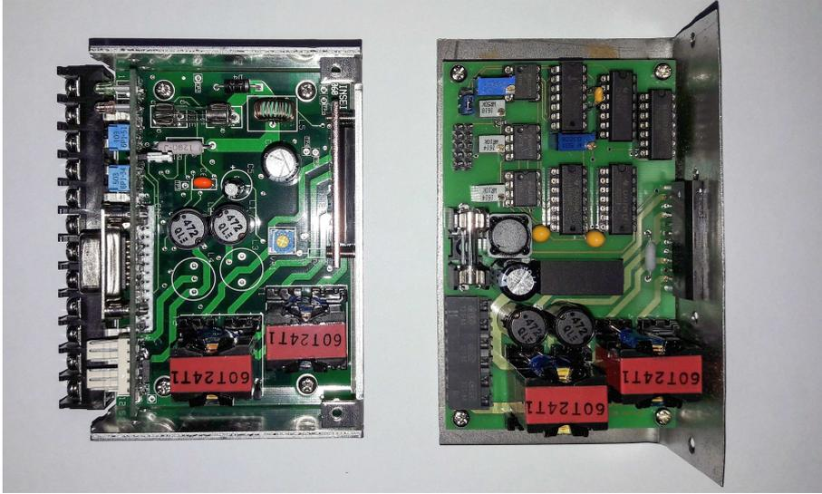
Figure 2.6: Photograph of the original (left) and modified (right) motor driver.
