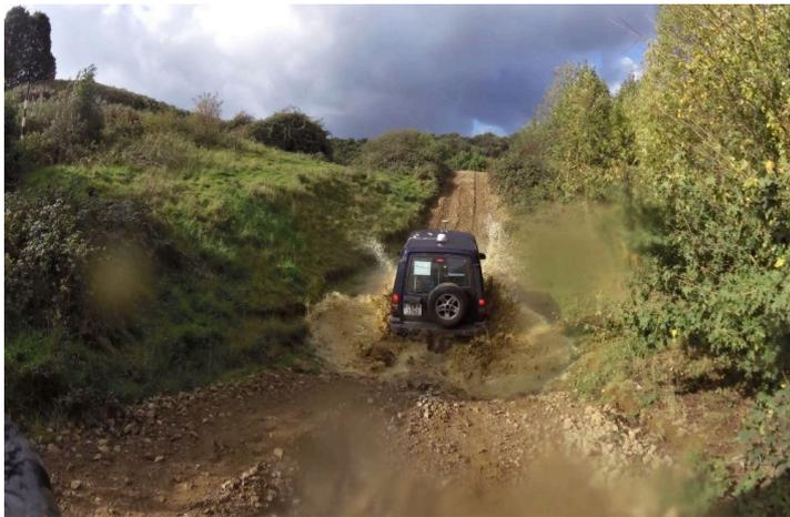
**Figure 5.1:** A measurement with an off-road vehicle in the Millbrook Proving Ground (MPG). The vehicle is in a deep ditch designed to test the dynamics in such an off-road scenario.
