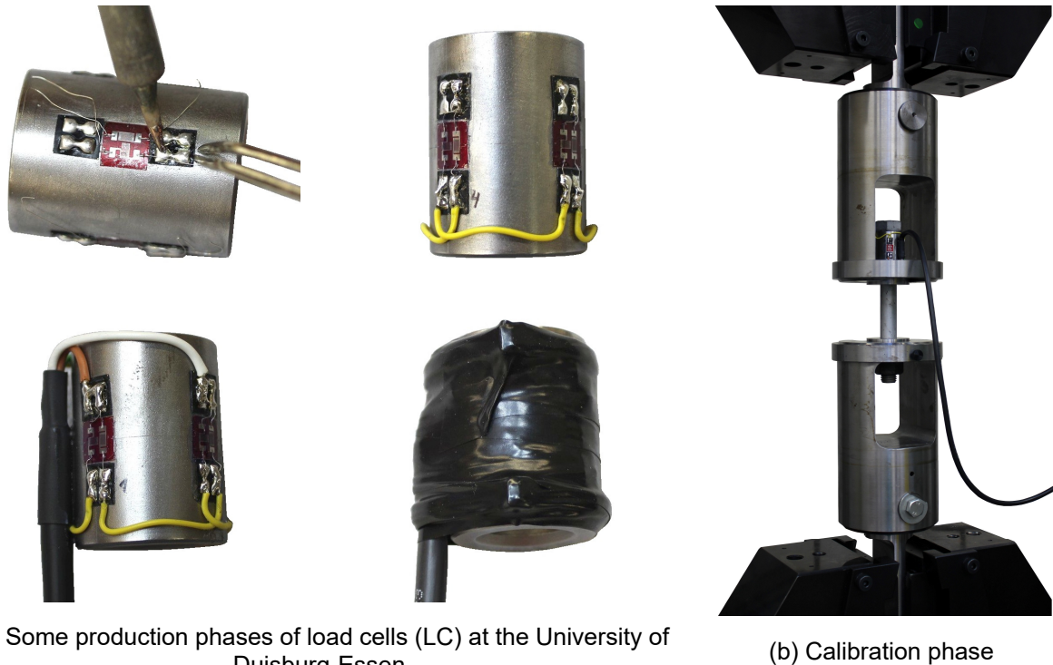
Figure 4-11: Preparation and calibration phases of load cells
