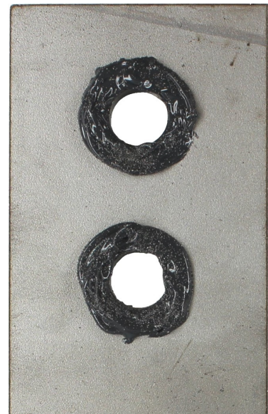
(c) Surface around the hole was covered with thick layer of resin and partially covered with particles (thhR+pP)
