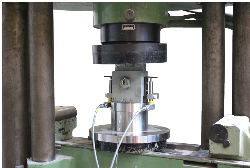
Figure 6-5: Testing adapter in order to perform the static tests according to RCSC, Appendix A
