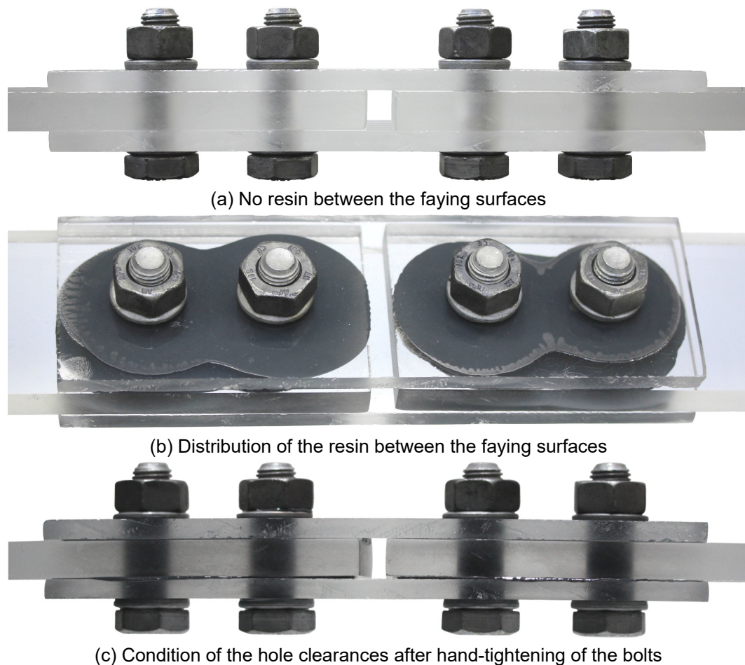
Figure 5-29: Condition of the hole clearance without and with resin between the faying surfaces
