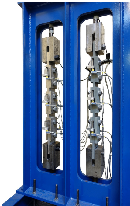
(a) Test chain setup according to RCSC, Appendix A
