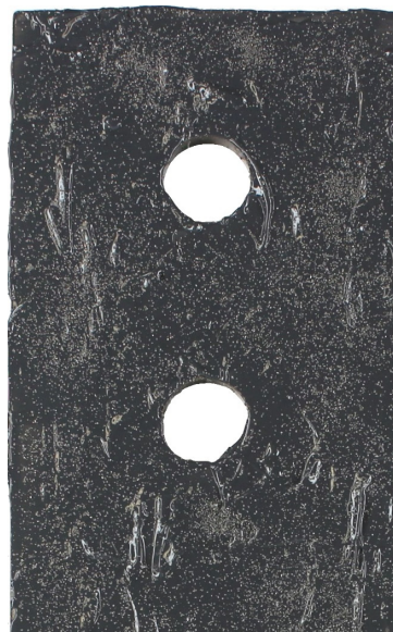
(b) Surface was covered with thick layer of resin and partially covered with particles (thR+pP)
