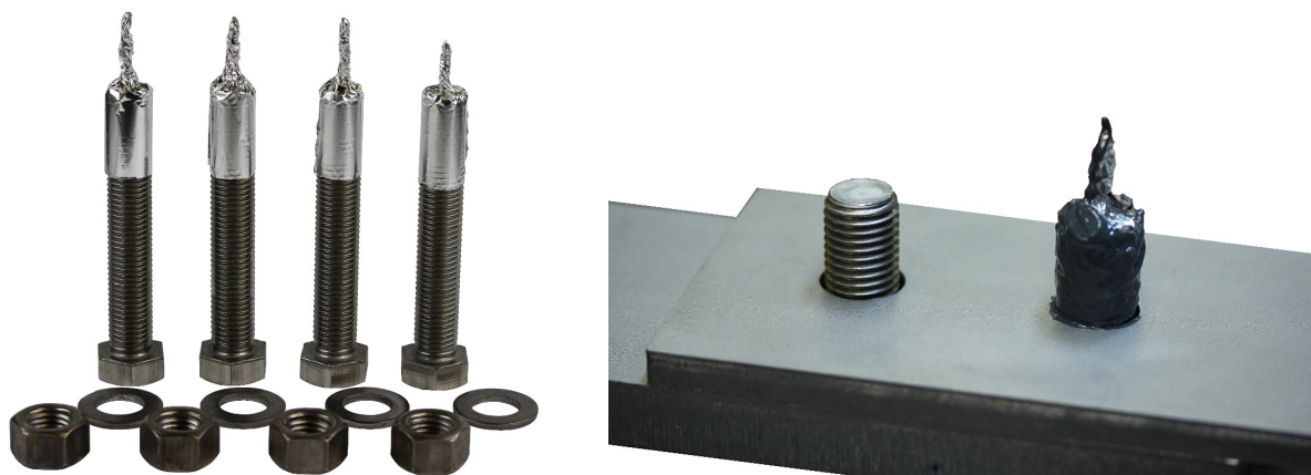
Figure 5-21: Using aluminium cap to protect the thread of the bolts
