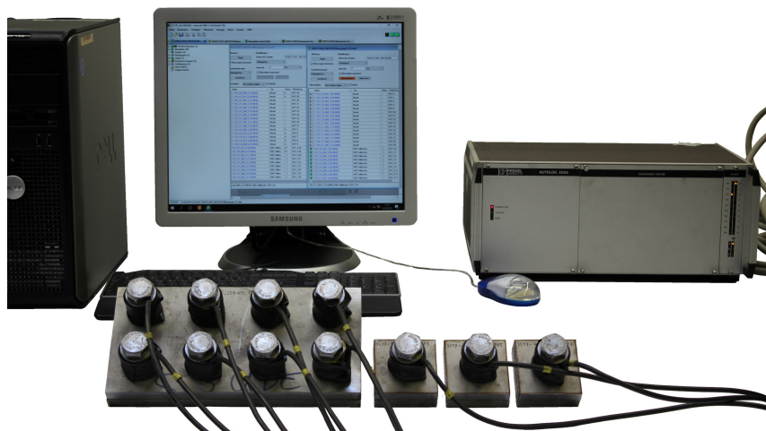
(c) Preload in the bolts continuously measured during the tests
