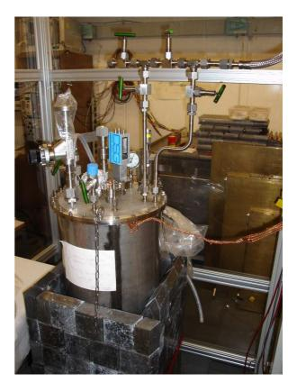
Figure 4.3: The closed LArGe@MPI-K system. Right: the flushing tubes. Middle: the preamplifier. Bottom: the unfinished lead shielding.
