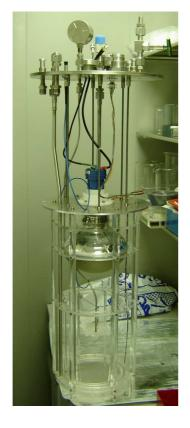
Figure 4.2: The inner part of the LArGe@MPI-K system. From top to bottom: stainless steel lid, aluminium lid, PMT, source-tube and acrylic mounting structure for WLS and diode.
