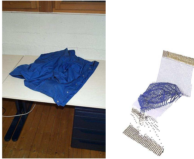
Figure 5.10: A blue jacket lying on a desk. Photograph of the scene (left) and 3D scan with color information added. The example is used to evaluate the color-based plane extraction. Comparing the plane extracted for the table top, we obtain an improved estimate over the non-color based plane extraction (see text).
