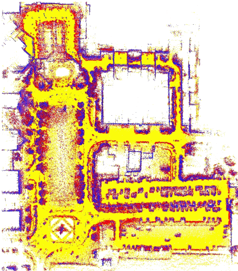
a. Top view of the resulting MLS map with a cell size of 50 \times 50 cm. The yellow surface patches are classified as traversable.
