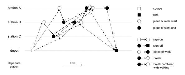
Figure 3.2.: Time-space duty generation network
