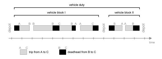
Figure 1.3.: Schedule of one vehicle consisting of two blocks
