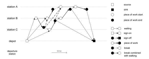
Figure 3.3.: Aggregated time-space duty generation network
