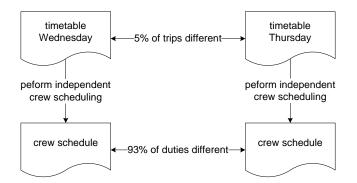
Figure 1.8.: Impact of an irregular timetable on the regularity of the crew scheduling solution if independent crew scheduling is performed.
