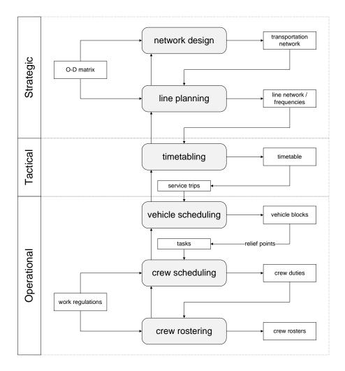
Figure 1.1.: Planning Process of a Public Transport Company
