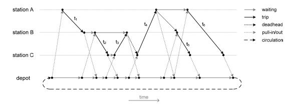
Figure 2.3.: Time-space network with six trips
