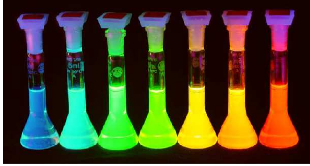
Figure 1.1.: Luminescence from colloidal quantum dots of different size and composition. The peak wavelength of the emission can be tuned all the way through the visible range of the optical spectrum and farther into the infrared. Courtesy of Dr. Andrey Rogach [1].
