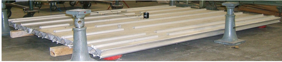
Figure F.23: Photo of test set-up, suspension by air-filled balls in red
