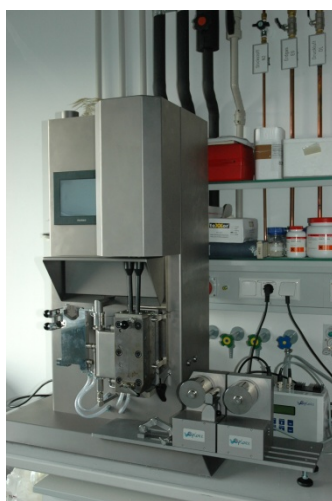
Figure 40: X-plore extruder for the production of polymer films
