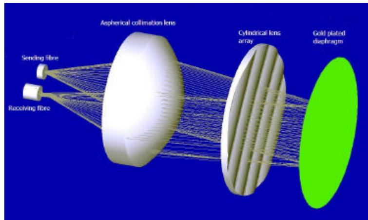
**Figure 9** The confocal optical microphone
