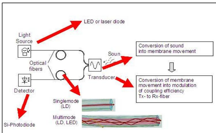
Figure 7 Schematic of the optical transducer
