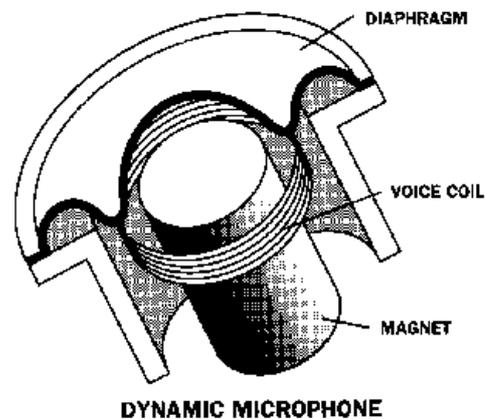
Figure 2 Schematic design of the dynamic microphone
