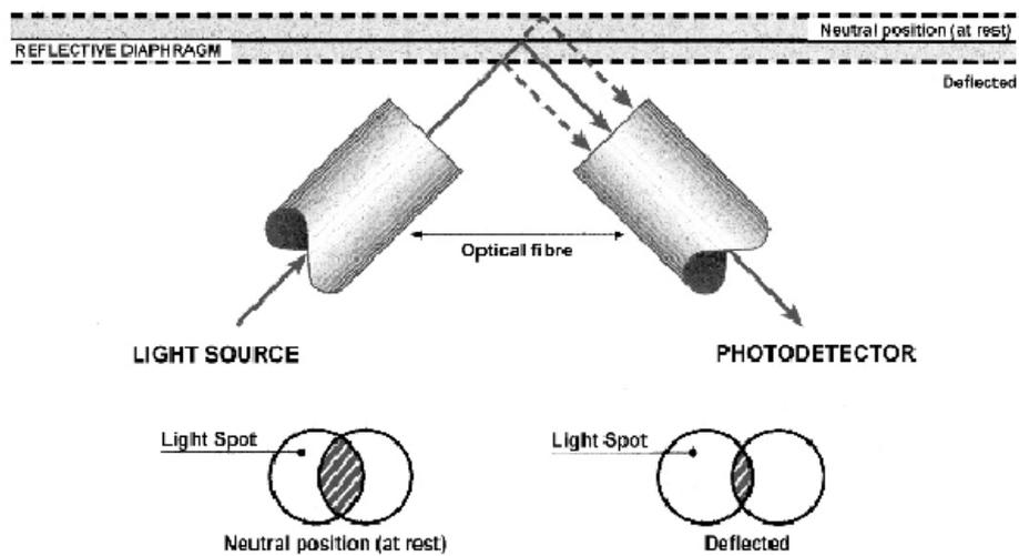
**Figure 12** The image shifting optical microphone
