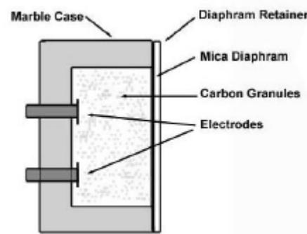
**Figure 1** Schematic of the carbon microphone
