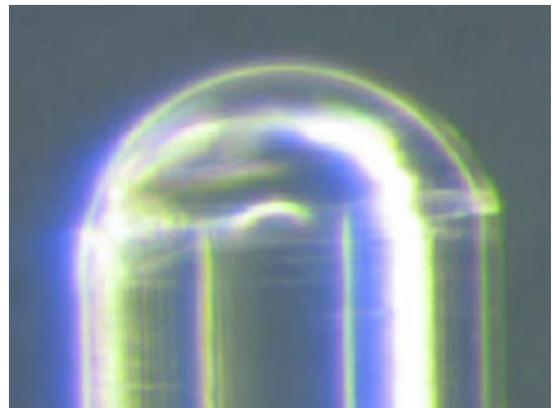
**Figure 13** The polymeric lens on the sending fibre
