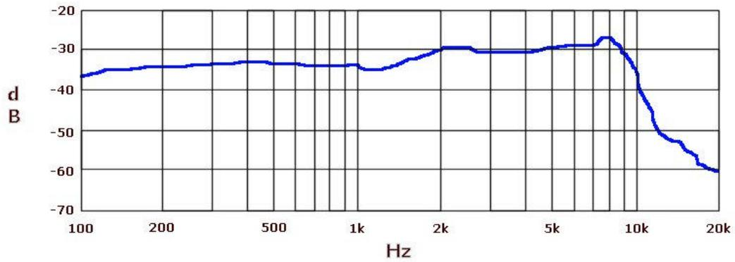
**Figure 10** Frequency response of the confocal optical microphone without any response correction dampening in place.
