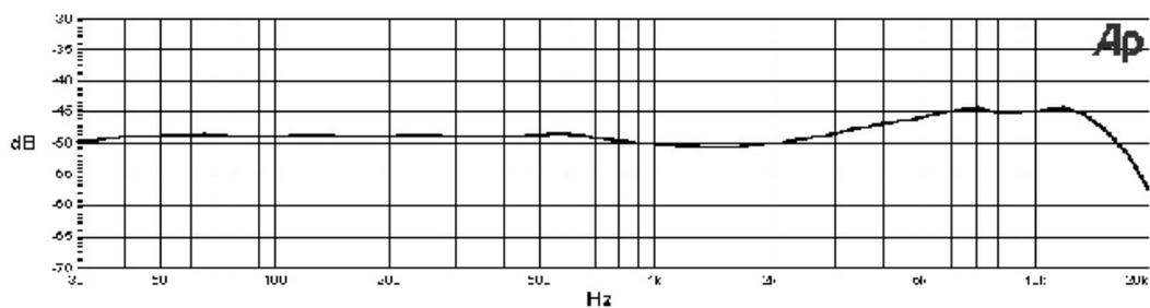
Figure 15 Frequency response of the image shifting design by Sennheiser.
