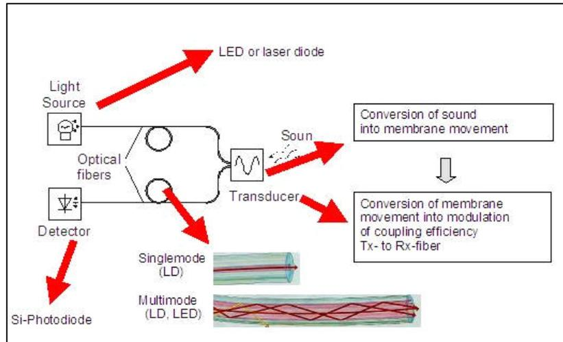
**Figure 17** Schematic of the optical microphone
