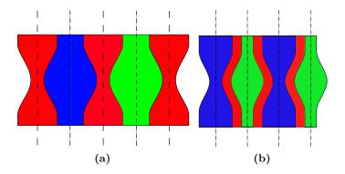
**Figure 4.17.:** Predictions of oscillatory modes for the  $\alpha\beta\alpha\gamma$  arrangement, reminiscent of the 1- $\lambda$ -O mode (a) and 2- $\lambda$ -O mode (b) in binary eutectics.
