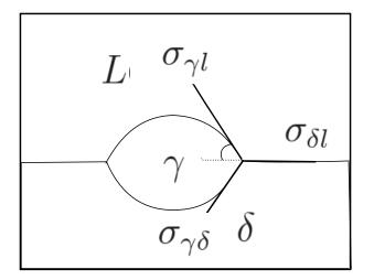
Figure 3.10.: Illustration of the angle that the surface tangent at the  $l - \delta$  interface close to the triple junction, makes with the horizontal (original substrate).
