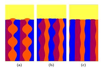
Figure 4.14.: Oscillatory modes in simulations for the  $\alpha\beta\gamma$  configuration at the off-eutectic concentrations  $\boldsymbol{c} = (0.32, 0.32, 0.36)$  in (a), and  $\boldsymbol{c} = (0.34, 0.34, 0.32)$  in (b) and (c). The spacings are  $\lambda = 170$  in (a) and (c) and  $\lambda = 165$  in (b).
