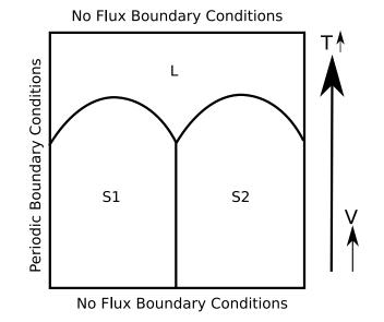
Figure 4.7.: Simulation setup for the phase-field simulations of binary and ternary eutectic systems. We impose a temperature gradient G along the z direction and move it with a fixed velocity. The average interface position follows the isotherms at steady state in case of stable lamellar coupled growth.
