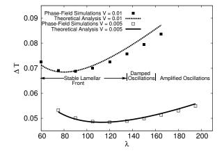
Figure 4.11.: Comparison between theoretical analysis and phase-field simulations at two different velocities for the arrangement  $(\alpha\beta\gamma)$  of ternary eutectic solids at V = 0.005and V = 0.01. The demarcation shows the regions of stable lamellar growth and the critical spacing beyond which we observe amplified oscillatory behavior. There is a small region named "Damped Oscillations", which is a region where oscillations occur but die down slowly with time.
