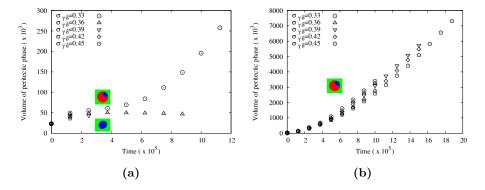
Figure 3.4.: Volume change of the peritectic  $\gamma$ -phase in time, illustrating the influence of the surface energy  $\tilde{\sigma}_{\gamma\delta}$  on the type of morphology and on the growth rate for two different concentrations (a)  $c_{Fe}^{l} = 0.95$  and (b)  $c_{Fe}^{l} = 0.97$  (Please read the legends in the graphs  $\sigma$  as  $\tilde{\sigma}$ )
