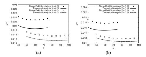
Figure 4.10.: Comparison of  $\Delta T - \lambda$  relations resulting from the theoretical analysis and from the phase-field simulations at two different velocities for systems; (a) symmetric binary eutectic system (A-B) and (b) unsymmetric binary eutectic system (C-D).
