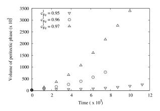
**Figure 3.2.:** Growth of the peritectic  $\gamma$ -phase during engulfment, for different concentrations  $c_{Fe}^{l}$  of the liquid phase and for a constant surface energy  $\tilde{\sigma}_{\gamma\delta} = 0.33$
