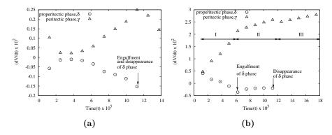
Figure 3.3.: Rate of volume change of the peritectic and properitectic phases with time for a constant surface energy  $\tilde{\sigma}_{\gamma\delta} = 0.33$  and for two different liquid concentrations (a)  $c_{Fe}^{l} = 0.95$  and (b)  $c_{Fe}^{l} = 0.97$ .
