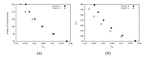
Figure 3.8.: Calculation of the radius of the critical profiles for homogeneous nucleation at T=0.97 in a) and barrier to nucleation in b).
