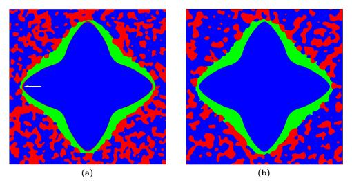
Figure 3.6.: Phase-field simulations of nucleation in the peritectic Fe-C system for two different surface energies  $\tilde{\sigma}_{\gamma\delta} = 0.39$  and  $\tilde{\sigma}_{\gamma\delta} = 0.778$  in comparison. (a) For the lower value of the solid-solid surface energy, heterogeneous nucleation can be seen at the dendrite tips, (b) For the higher value, the nuclei are purely formed homogeneously in the liquid. Color coding; Red:  $\gamma$ - phase, Blue:  $\delta$ -phase, Green: Liquid
