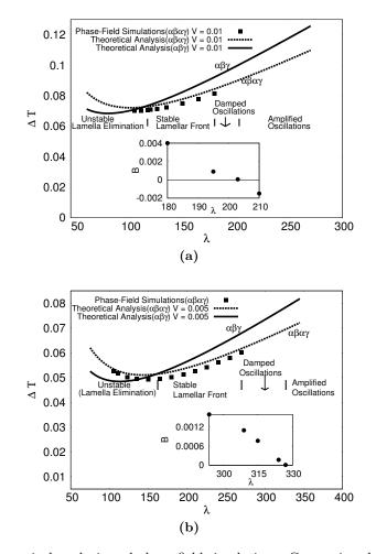
Figure 4.16.: Theoretical analysis and phase-field simulations: Comparison between the arrangements  $(\alpha\beta\gamma)$  and  $(\alpha\beta\alpha\gamma)$  for two different velocities (a) V = 0.005 and (b) V = 0.01. Plots convey information on the stability ranges, and the onset of oscillatory behavior of the 1- $\lambda$ -O type.
