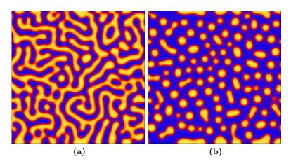
Figure 2.3.: Phase separation at two different compositions of the liquid in a model Fe-Sn alloy. In (a) the simulation is performed at the monotectic composition while in (b) a hyper-monotectic composition is employed.(Work along with co-worker Wang Fei)
