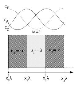
**Figure 4.4.:** Sketch of a ternary stacking order  $(\alpha\beta\gamma)$  with period length M = 3.
