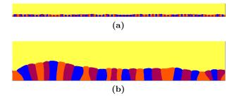
Figure 4.23.: Two snapshots of 2D dynamics in a large system. Isothermal simulations are started from a random configuration in (a) where the probability of occurrence of each phase is 1/3, which is also the global concentration in the liquid. The temperature of the system is T=0.785 and the concentration of the liquid is the eutectic concentration. A slowly changing pattern with a non-planar front is achieved. Some lamellae are eliminated, but no new lamellae are created.
