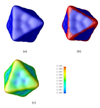
Figure 3.7.: Phase-field simulation of a dendritic microstructure with four-fold surface energy anisotropy: (a) final shape of the properitectic phase, (b) heterogeneous nucleation at the edges and tips of the dendrite and (c) concentration of Fe at the dendritic surface for the same time step as in (b).
