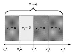
Figure 4.5.: Schematic drawing of a ternary eutectic system with a configuration  $(\alpha\beta\alpha\gamma\alpha\beta\ldots)$  of periodic length M = 4.
