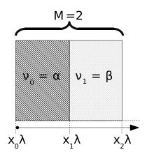
Figure 4.3.: Sketch of a lamellar structure in a binary eutectic system with period length M = 2.  $\nu_i$  denotes a phase in the sequence  $(\alpha\beta)$ .
