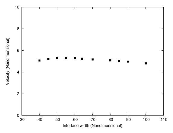
Figure 5.1.: Velocity of a pure nickel planar front simulated with different  $\varepsilon$  at a fixed nondimensional temperature of T=0.96.
