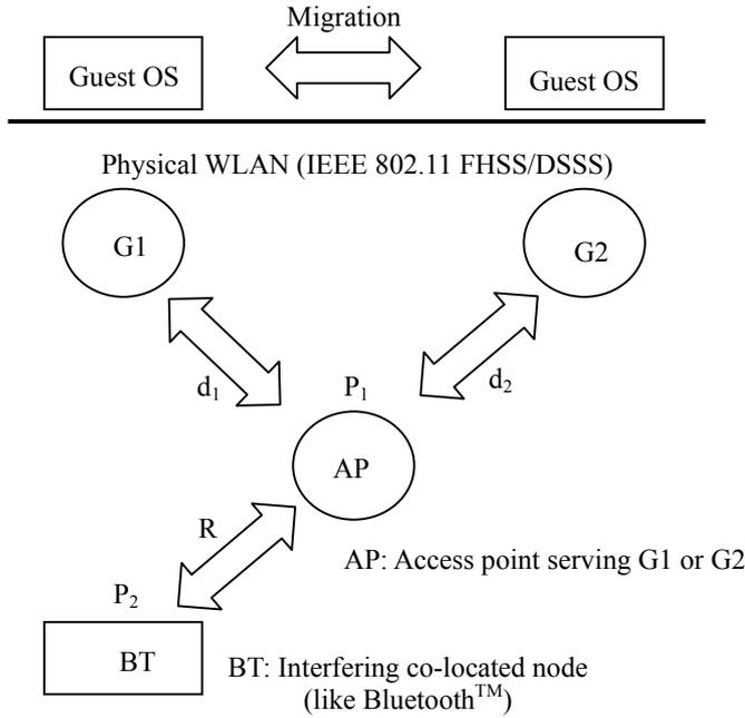
**Figure 2:** An interference scenario of OS migration set on a WLAN-link. The RF interference (RFI) is presumably caused by an IEEE 802.11 FHSS/DSSS device (like Bluetooth™) communication.  $R$ ,  $d_1$ , and  $d_2$  are node separations (in meter) as shown,  $P_1$  and  $P_2$  are transmitted power levels of the units.
