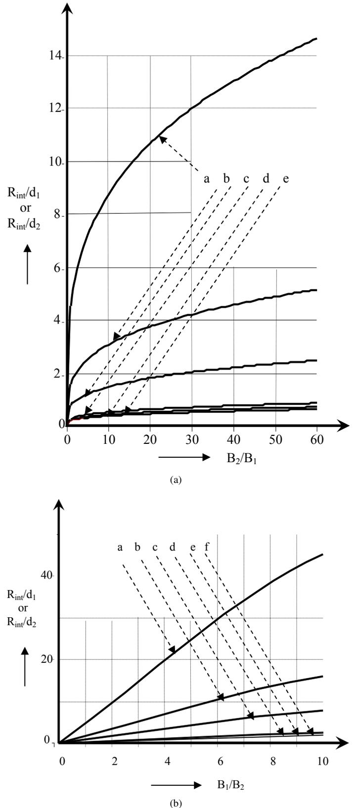
**Figure 4:**  $B_1/B_2$  ratio ( $>1$ ) versus  $R_{\text{int}}$  (normalized with respect to  $d_1$  or  $d_2$ ) for a set of parametric values of the probability of bit-error (BER). The graphs shown correspond to  $P_e = \{0.0001, 0.0010, 0.0050, 0.0500, 0.0750, 0.1000\} \equiv \{a, b, c, d, e, f\}$ ; (a)  $B_2/B_1$  ratio over a range of 0 to 600, (b)  $B_1/B_2$  ratio over a range of 0 to 10.
