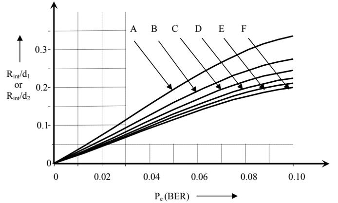
**Figure 3:**  $R_{int}$  (normalized with respect to  $d_1$  or  $d_2$ ) *versus* the probability of bit-error (BER) for a set of parametric values,  $B_1/B_2$ . The graphs shown correspond to the following sets:  $B_1/B_2 = \{1/100, 1/200, 1/300, 1/400, 1/500, 1/600\} \equiv \{A, B, C, D, E, F\}$ .
