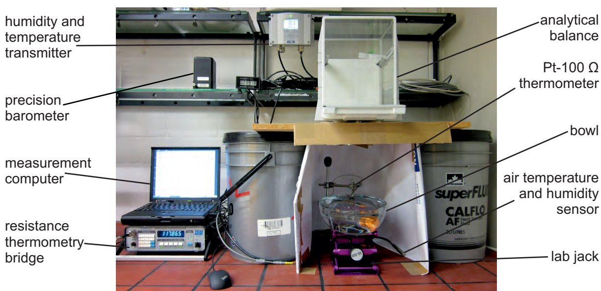
Figure 4.12 Experimental setup for mass and volume calibrations.
