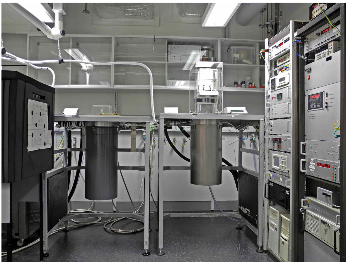
Figure 3.1 Photo of the low-pressure viscometer and the viscometer-densimeter in the new laboratory.
