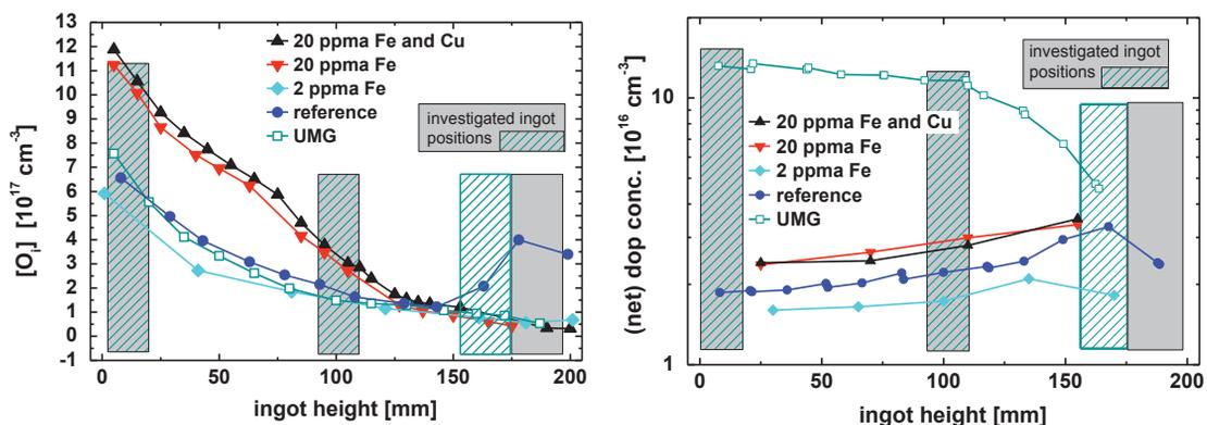
Fig. 2.  $[O_i]$  (left) and (net) dopant concentration (right) of the different investigated materials over the ingot height (as grown).
