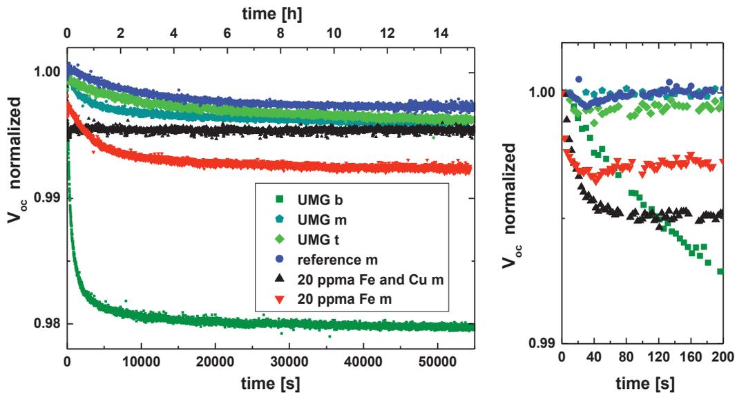
Fig. 3. Time resolved evolution of the  $V_{oc}$  decay of solar cells made from different materials under 1 sun illumination at 25°C. The left side shows the decay for all materials during 14 h of illumination at 1 sun. The very fast decay for Fe and Fe/Cu contaminated material (originating from the middle of the respective ingot) is depicted on the right side (same data but different time scale).
