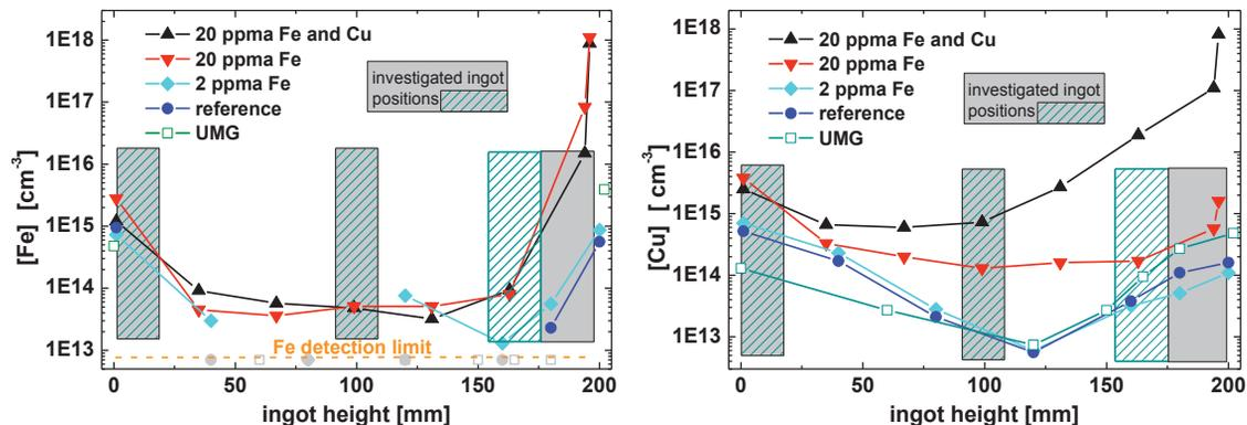
Fig. 1. Height distribution of [Fe] (left) and [Cu] (right) for the investigated materials (as grown). The approximated positions where the material for solar cell processing is taken from are marked in grey (or shaded green for the UMG material).
