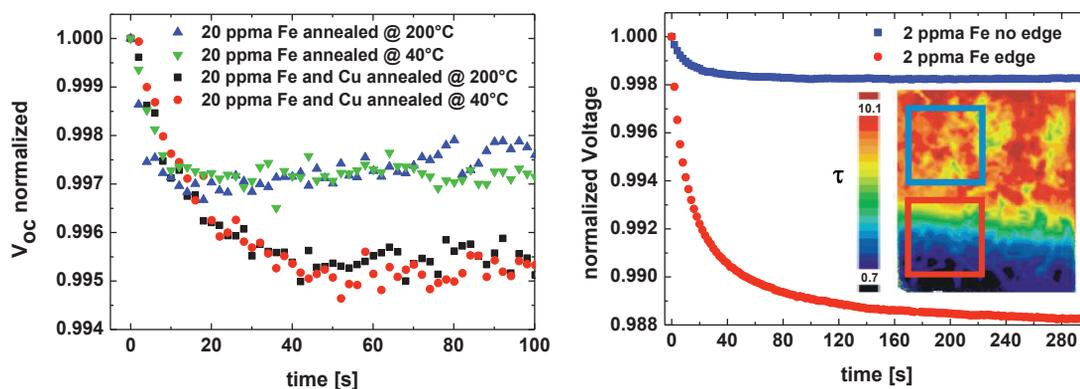
Fig. 4. Time resolved degradation of Fe/Cu and Fe contaminated material after different annealing steps (left) and influence of the crucible wall on degradation (right). The origin of the investigated test cells is marked in the inserted lifetime map of the as grown wafer and colors are analogous to the graph's colors.
