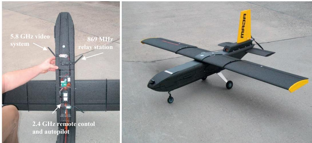
**Fig. 2:** Image of the relay station MAJA and the different radio systems.
