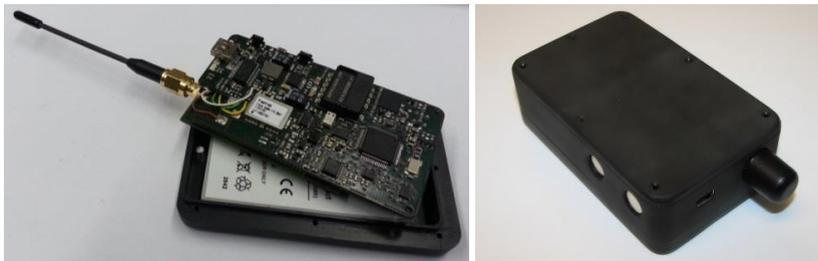
Fig. 1: BodyGuard (BG)-System Version 2.0, left: the board of the BG-System with the used sensors, right: BG-System ready for action.
