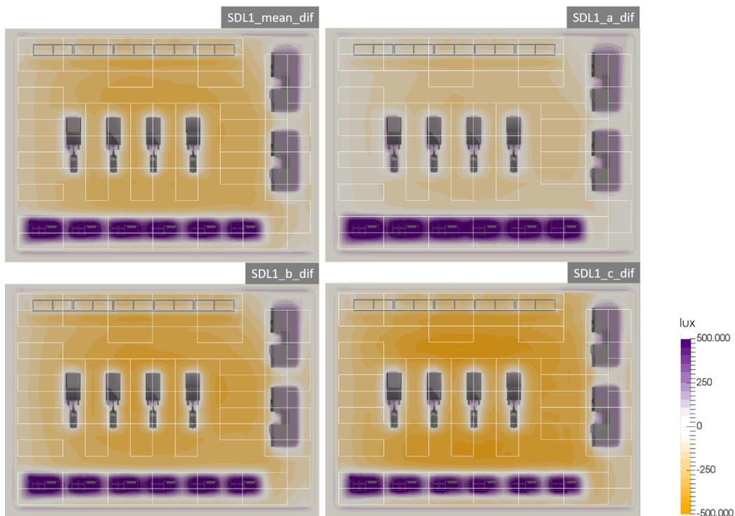
**Fig. 3.13.:** Comparison of simulation results for SDL1 against the minimum requirement grid.
