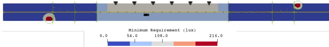
**Fig. 3.22.:** Minimum illuminance requirement grid for modeled road work zone.
