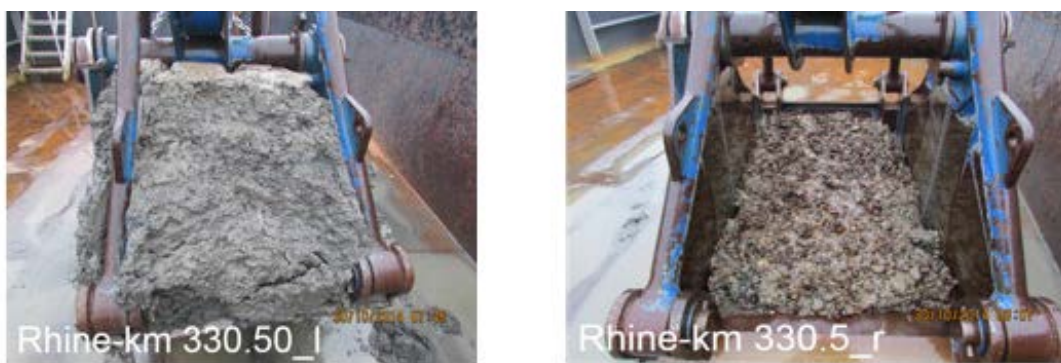
Figure 3.6: Observed sediment grain size at Rhine-km 330.5 at the left and right hand side, 500 m downstream of the upstream model boundary (BfG, 2014).
