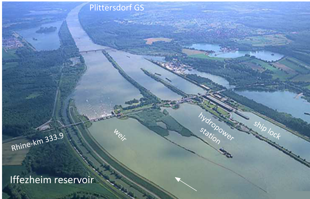
Figure 1.2: Iffezheim reservoir and Plittersdorf gauging station in the downstream (modified from Köthe et al. (2004)).
