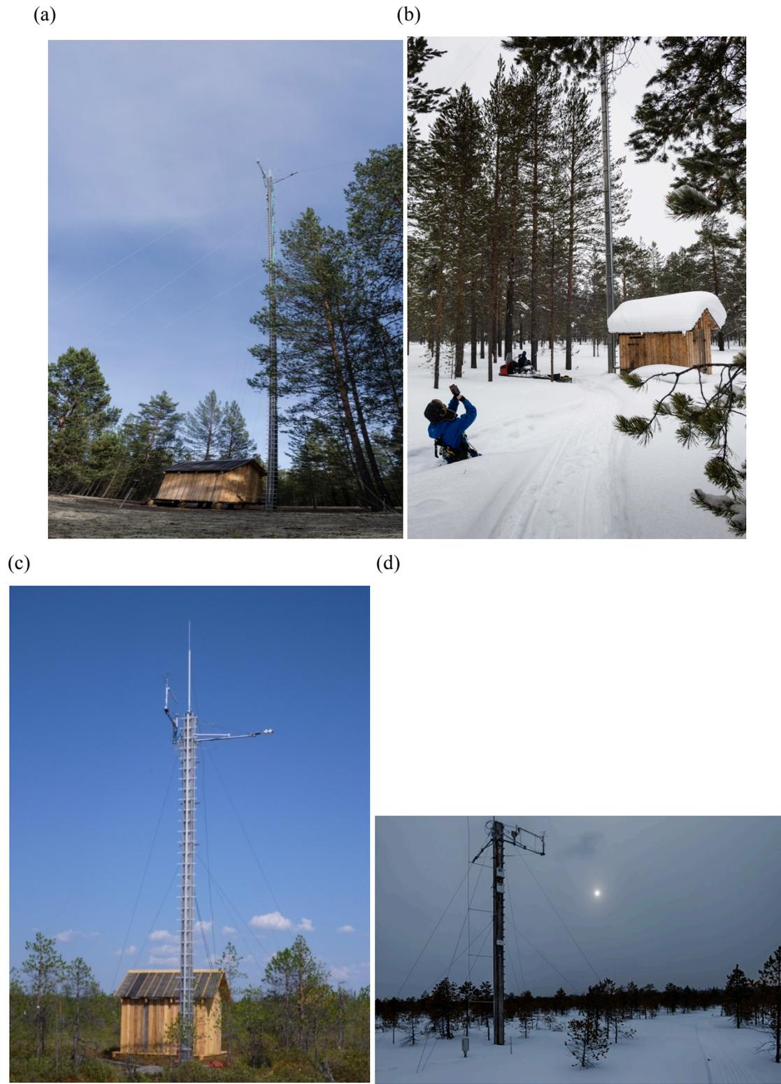
Figure 4.2 Eddy covariance flux towers (a) at the Zotino Forest (ZF) site in growing season and (b) snow season and (c) Zotino Bog (ZB) site in growing season and (d) snow season. The measurement heights are 30.3 m and 9.9 m, respectively. Details of the instrumentation are shown in Table 4.2.
