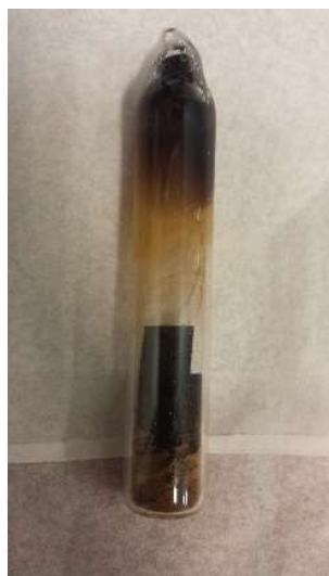
Figure A4: Ampoule prior to opening. The CMB complex, which initially had no color, has turned brown during the reaction. The nickel foam shows a black brown color after to reaction (compared to metallic before). A black, brownish accumulation of material, partially containing crystals, is found at the top of the ampoule.
