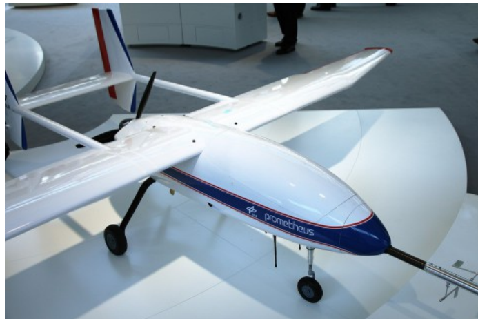
Figure 4.5: Prometheus Fixed Wing UAV [www.dlr.de]
