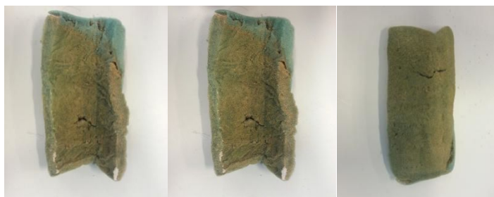
Fig.2.2 Polyethylene sponges after adsorption of cells.
