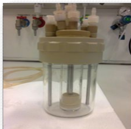
Figure 1.4b. Packed Bed Bioreactor from Medorex.e.K
