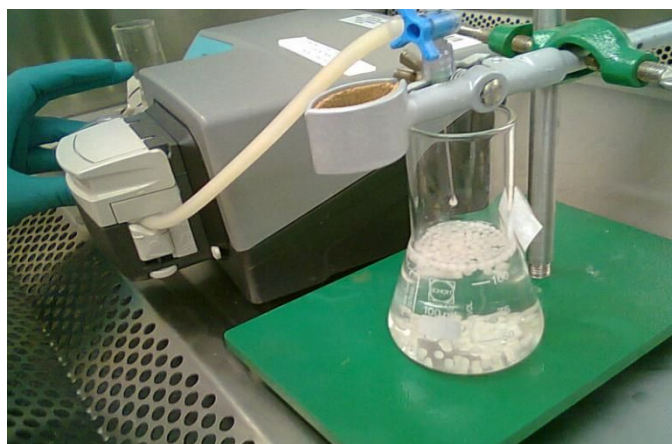
Figure 2.1. Alginate beads preparation
