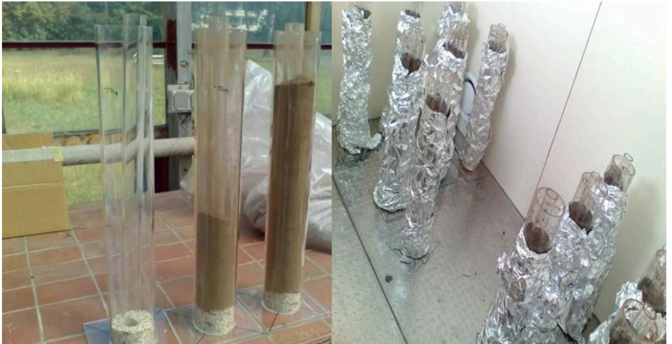
**Figure S2.3:** The microcosm design and structure (Left). The aluminum foil wrapped microcosms (Right).
