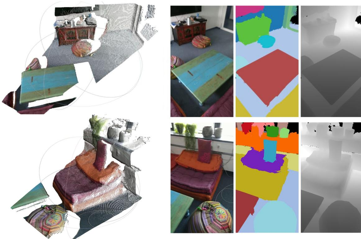
**Fig. 3.1.** Example of a 3D scene pair of the *RIO* dataset [295]. It provides a) registered, texture-mapped 3D reconstructions, c) dense instance-level semantic segmentation and symmetry-aware transformations of rigid changes as well as c) calibrated RGB-D sequences.
