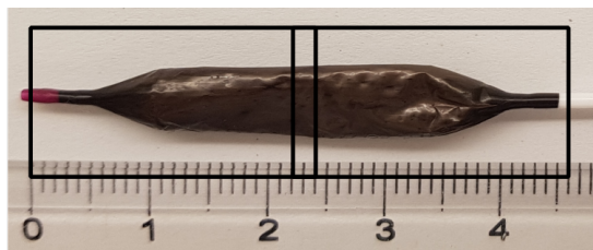
Figure 1: Picture of the balloon catheter together with a sketch of the measurement areas used in the multi-patch experiment.
