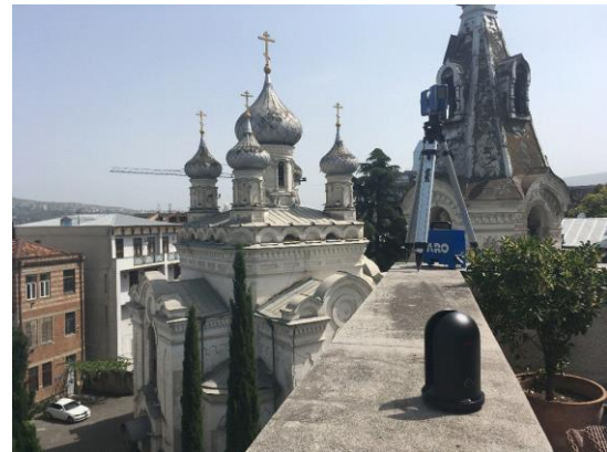
Figure 2. Russian-orthodox church in Lurdji complex; in foreground: Leica BLK360; in background: Faro scanner
