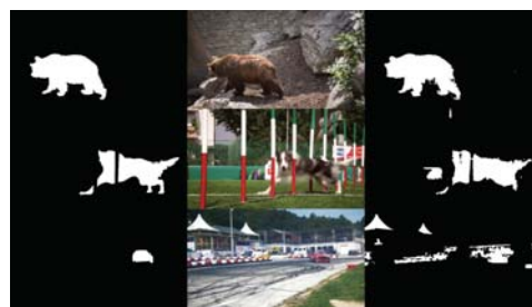
Fig. 3. Ground truth mask (left), input frame (middle) and predicted mask (right) for the bear , dog-agility and drift-straight sequences of DAVIS2017.
