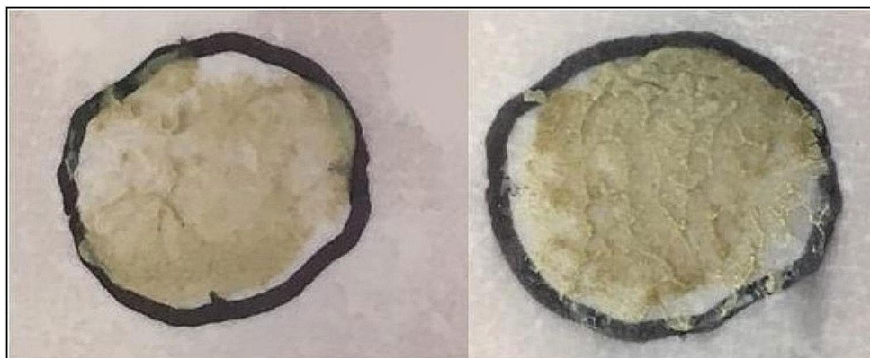
Fig. 2 Evaluation of sample quantities on the biological membrane (left: \cong 17.4 mg; right: \cong 30 mg)
