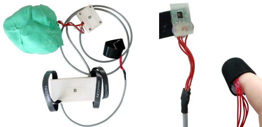
Figure 5: One complete PiHeart prototype including both units enclosed in 3d printed cases and the servomotor inside the silicon heart is shown on the left. On the right the heart rate sensor with Velcro and silicon protection is visible in detail.
