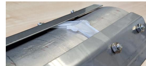
Environmental stress cracking test
