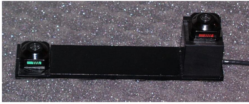
(a) Tracking unit (two beacons + one inertial cube)
