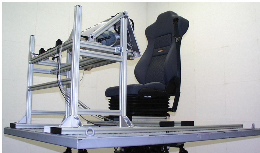
Figure 2.20: Driving setup with force feedback steering wheel.
