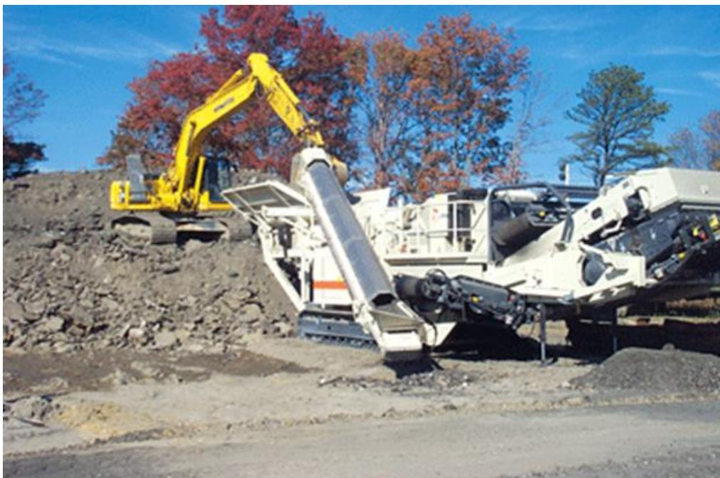
Figure 11 A mobile in- pit crusher [54]
