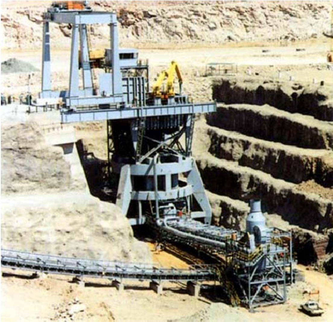
Figure 12 A semi-mobile in- pit crusher [54]
