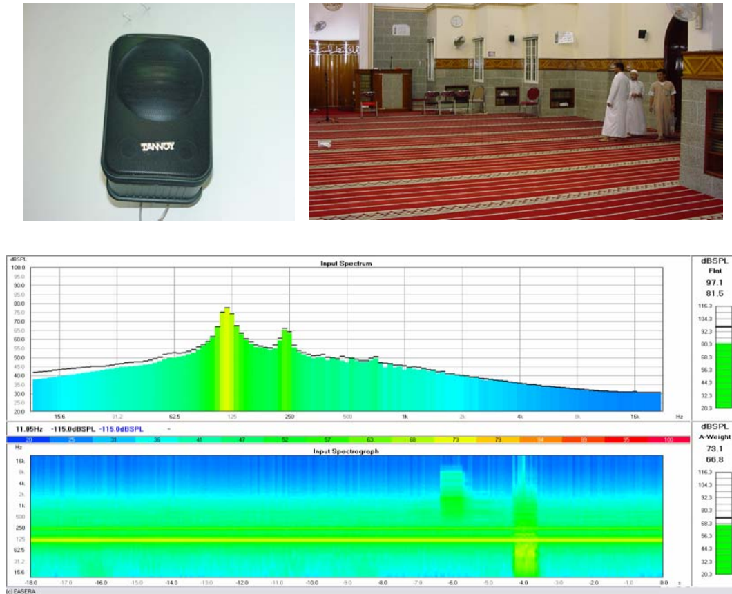
Figure 69. Internal view of Al-Eman Mosque and the measured BN spectrum at one of the measuring point
