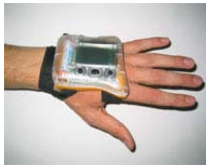
Figure 2.5 Pacemate sensor node
