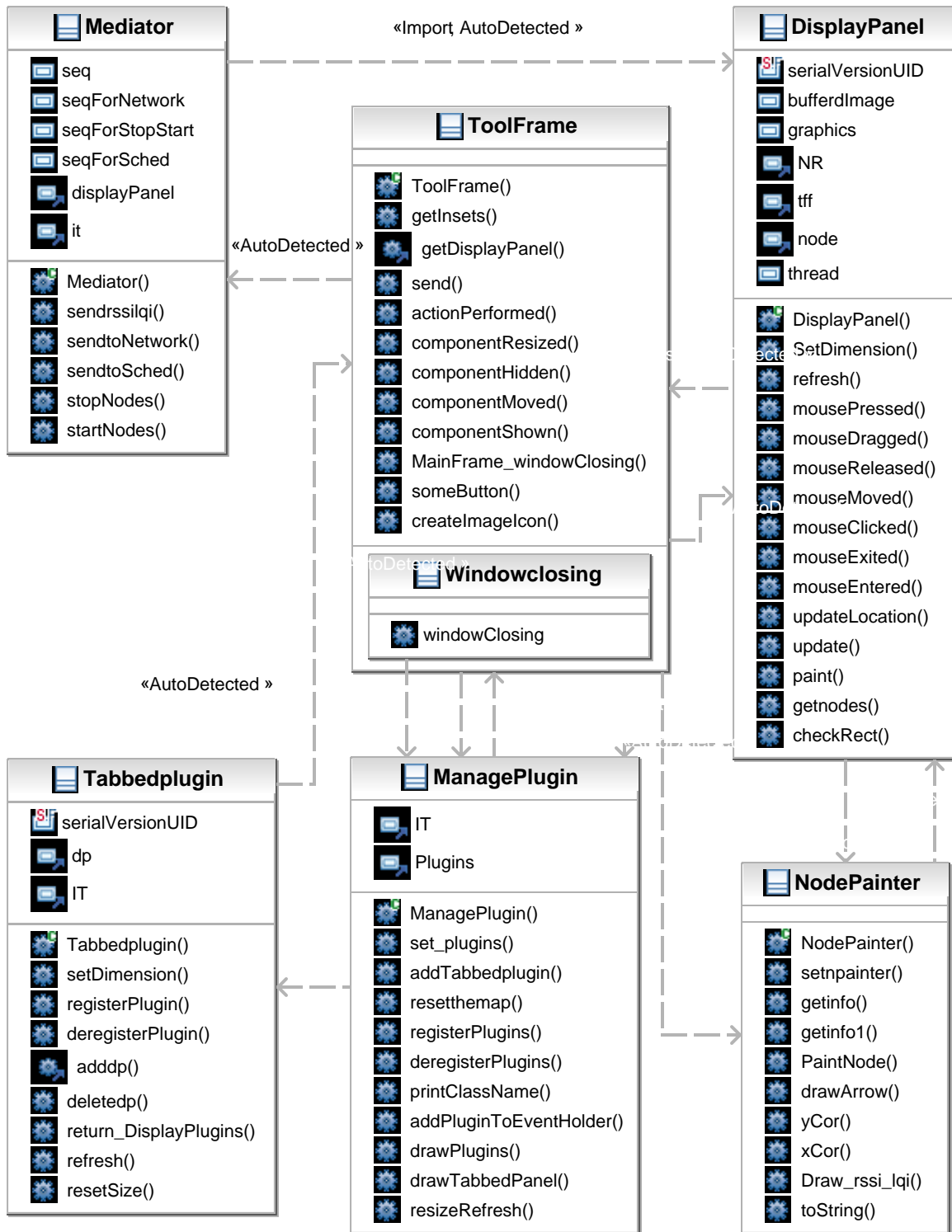
Figure 7.2 UML diagram of the visualization classes inside the management tool
